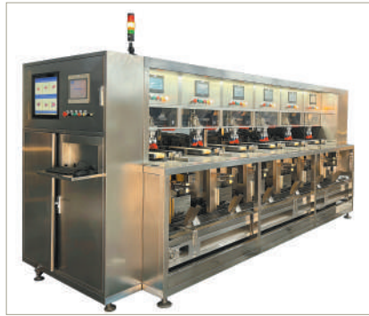
A fully automated AI-powered crayfish-peeling machine. (PHOTO: Ruifeng Intelligent Control Equipment Manufacturing Co., Ltd.)
