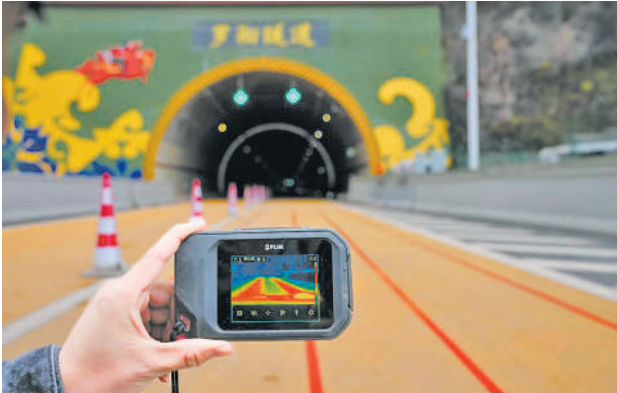
A staff member uses a thermal imager to test the effectiveness of the loop heat pipe snow melting system. (PHOTO: XINHUA)
