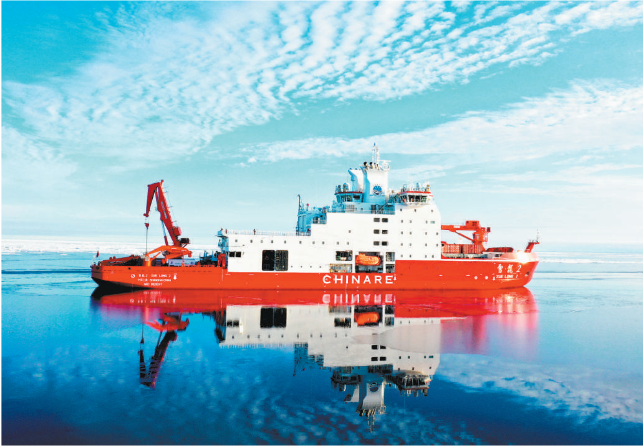
The photo shows Xuelong 2, which is China's first domestically built polar research icebreaker and the world's first icebreaker capable of breaking ice both bow-first and stern-first. (PHOTO:XINHUA)
