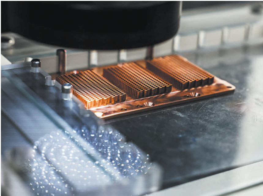
A new materials tech enterprise tests pin-type heat dissipation copper substrates. (PHOTO: XINHUA)
