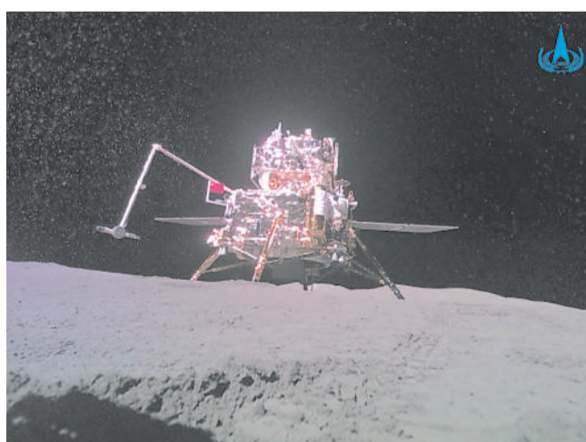
This photo taken by a mini rover released from the lander-ascender combination of Chang'e 6 probe shows a view of the combination itself on the lunar surface. (PHOTO: CNSA)
