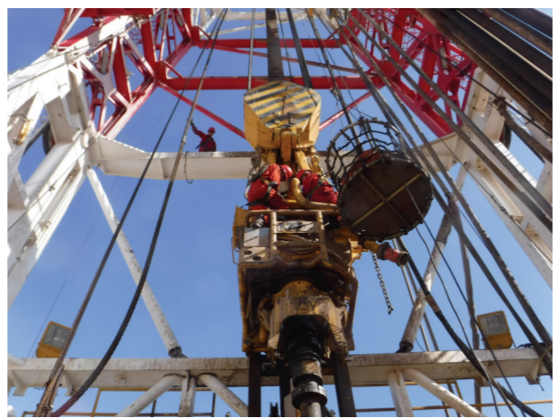
SP282完井后拆吊顶取
