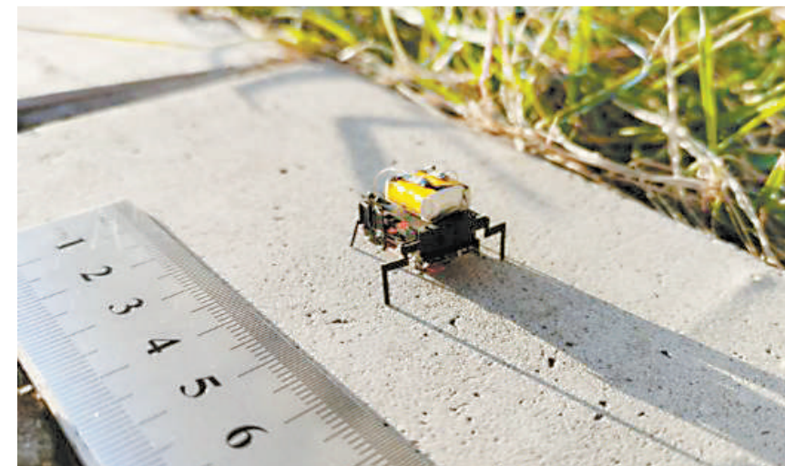
The BHMbot has a length of two centimeters. (PHOTO: Beihang University)
