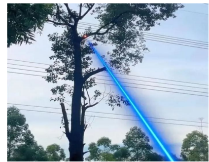
The laser obstacle remover trims the branches. (PHOTO: Red Coast Base Company)
